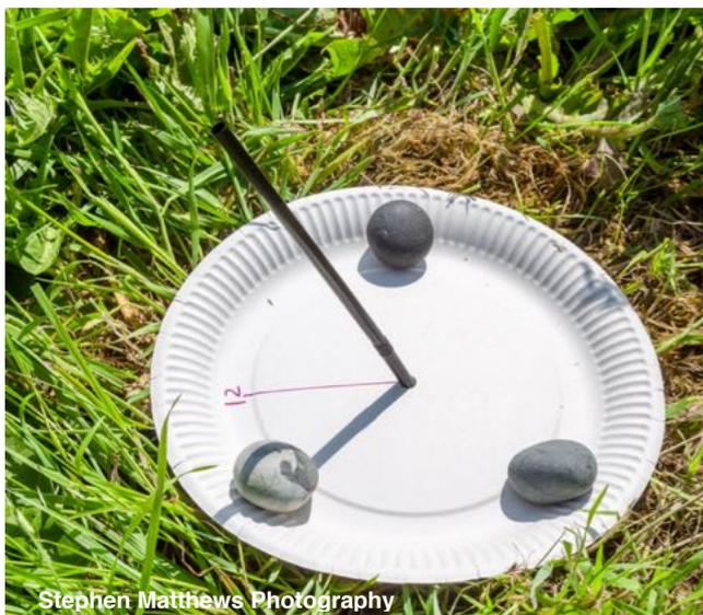
When it reaches 12 noon, rotate the plate so that the shadow from the stick falls across the number 12. You can then revisit the dial at different times to mark further numbers on. Test your clock over a few days (if dry!) Does the shadow from the sundial always tell the same time as your other clocks?
