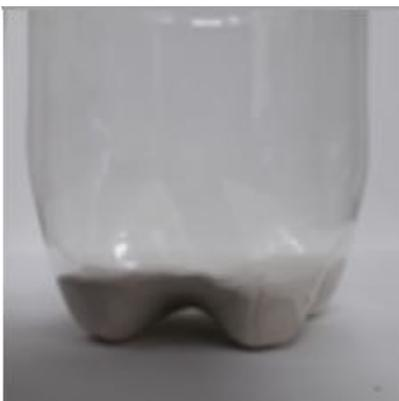
Use modelling clay to fill in the indentations in the bottom of the bottle, to give some stability and also to make the measurements more accurate.
